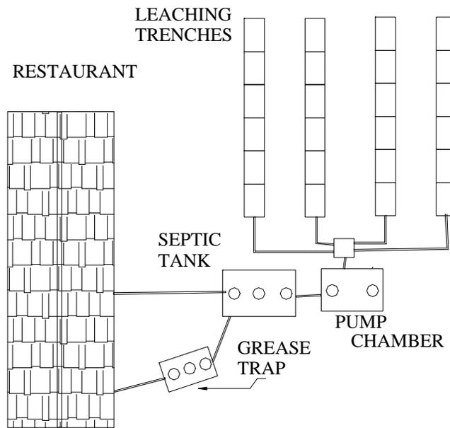
The structure of a grease trap is very similar to that of a septic tank with the exception of the sanitary tees. As can be seen in the illustration below, tees inside a grease trap penetrate
