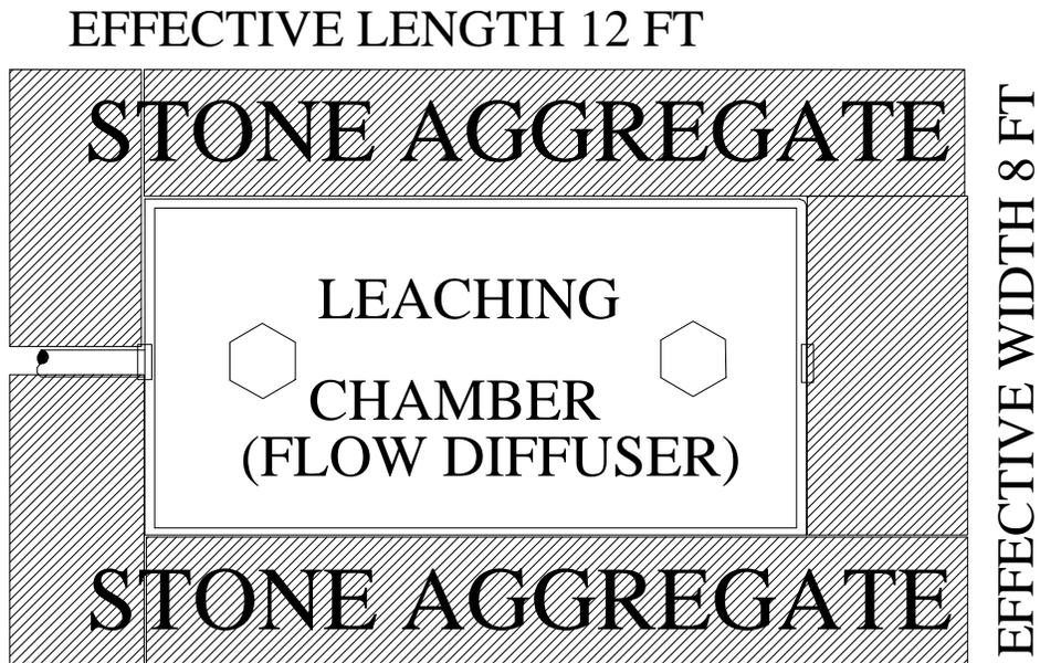
feet of stone surrounding the entire structure. In addition, the long sidewall area is 12' x 1', and the short sidewall area is 8' x 1'.
